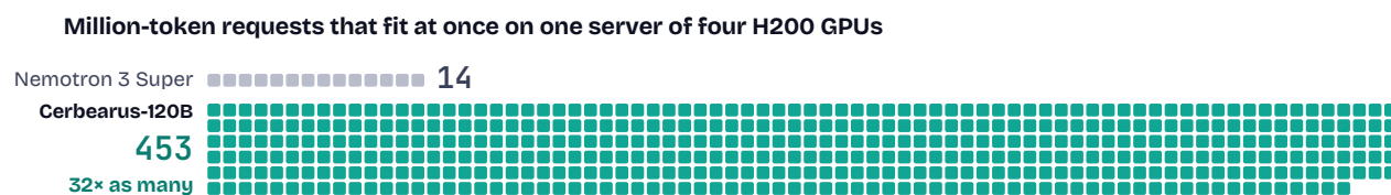
FIGURE 1 One server, four H200 GPUs. Each square is a million-token request held in memory at once.
